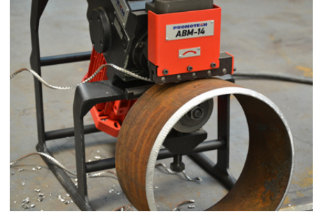
Oval workpiece and pipe beveling
