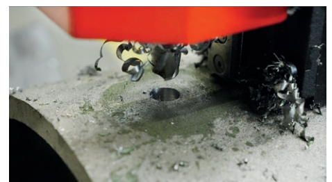
Max drilling capacity 16 mm
