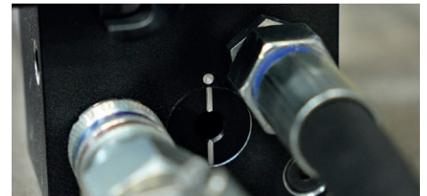
Clamping level indicator for safety and security
