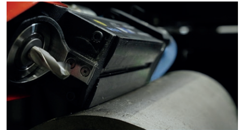
V-shaped prismatic mag base for pipe drilling
