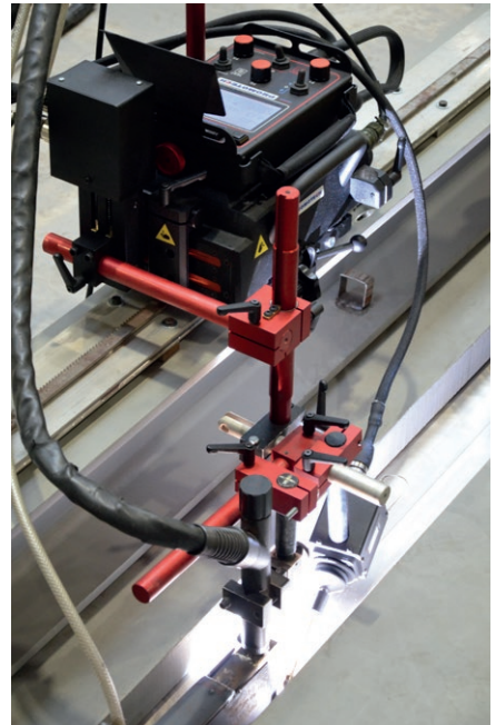
Seam tracking works with and without oscillation
