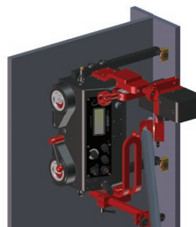
Fillet Welding with oscillator
