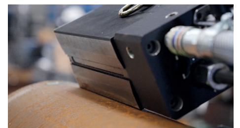
V-shaped prismatic mag base for pipe drilling
