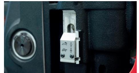
2-gearbox to match the speed to the tool
