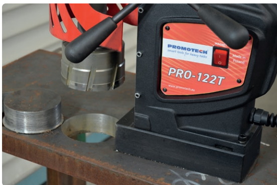
Milling capacity up to 120 mm (4-3/4")
