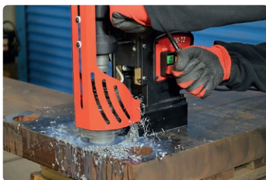
Milling capacity up to 70mm (2-3/4")
