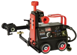
GECKO • Continuous welding • Dual torch welding
