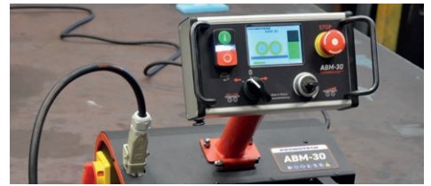
Control panel indicates current work mode and gives safety and diagnostic information
