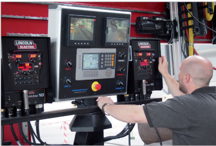
Sample view of CB operating panel and integrated SAW ACDC welding equipment from (Lincoln Electric and ESAB)
