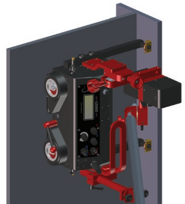
Fillet Welding with oscillator
