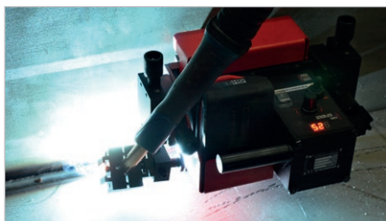
Torch placement on either side
