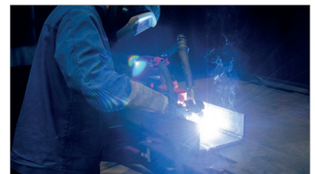
Welding in narrow spaces (min. width 200 mm)
