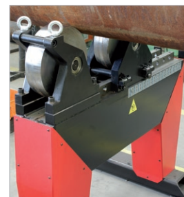
Heavy-duty adjustable pipe support (Ø 200-1000 mm)
