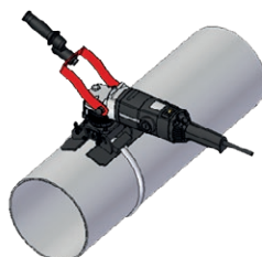
Attachment for removal of welded joints from longitudinal and circumferential surfaces (min. OD 200 mm, min. ID 400 mm) with angle adjustment from -10 to +30 degrees tanged to the cylindrical surface.
