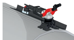
Attachment for removal of welded joints from longitudinal and circumferential surfaces (min. OD 200 mm, min. ID 400 mm) with angle adjustment from -10 to +30 degrees tanged to the cylindrical surface.
