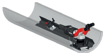
Attachment for removal of welded joints from longitudinal cylindrical surfaces (min. ID 350 mm) with tilt angle adjustment up to 15 degrees.
