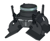
Attachment for removal of welded joints from longitudinal and circumferential surfaces (min. OD 200 mm, min. ID 400 mm) with angle adjustment from -10 to +30 degrees tanged to the cylindrical surface.
