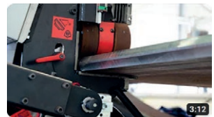
ABM 50 | Auto feed double-sided beveller 11K views • 5 years ago
