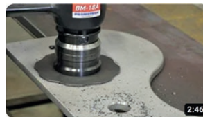
BM-18A | Pneumatic Plate Beveller 2.7K views • 3 years ago
