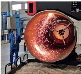
PPCM-1500 • 3D cutting/beveling oxy-fuel or plasma • Integrated library of macros • optional Lantek Flex3d Tubes software
