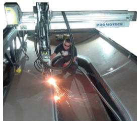
MCM-4000 • 5-Axis portable CNC 3D cutting & beveling and welding machines
